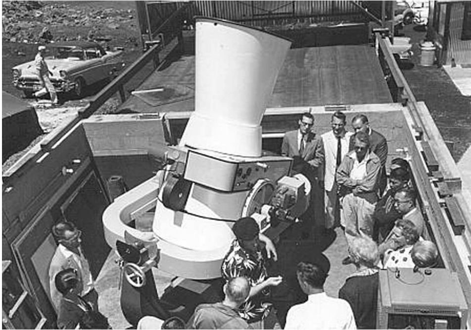
Figure 1. One of the twelve Baker-Nunn satellite-tracking cameras operated by the Smithsonian Astrophysical Observatory. This one, shown at its dedication on 2 August 1958, was located on the mountain of Haleakala on the Hawaiian island of Maui. Photo courtesy of Dr. Walter Steiger, University of Hawaii.
