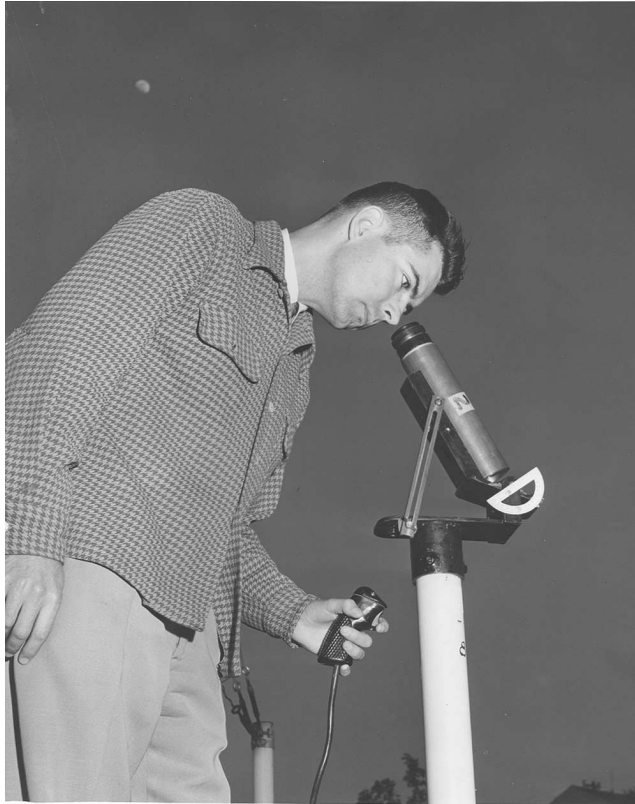
Figure 2. Donald Charles, a member of a Moonwatch team based in Walnut Creek, California, with a homemade Moonwatch telescope. Note the school protractor integrated into the mount, as well as the flat mirror in front of the telescope positioned to enable an observer to look down rather than up. The astronomer's hand holds a pushbutton device to mark passage of a satellite through his field of view. Photograph courtesy of Jack Borde.
