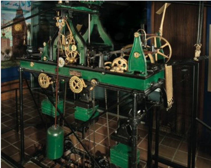
The 1929 clock that turns the hands on the courthouse tower.
